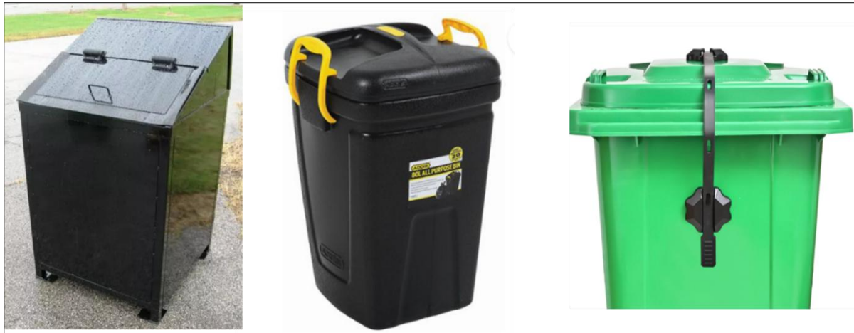
Figure 20. Wildlife-proof garbage disposal container options. Large containers with a one-way shoot to dispose of garbage (left): the top lid is connected to a smaller container which swivels up when the lid is opened to block access to the larger bin and its contents below, but when the lid is closed this bin swivels down to drop the garbage into the larger container. Locking mechanisms and handles on bins (middle and right) can also be used to successfully keep wildlife out.
