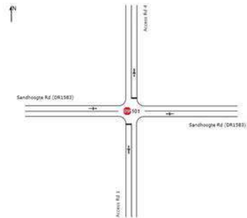
Figure 16: Geometry Intersection 1: Sandhoogte Rd (DR1583) / Development access 1 & 4
