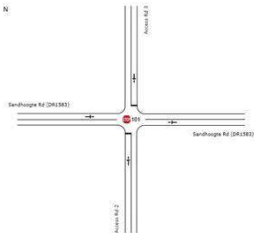
Figure 22: Geometry Intersection 3: Sandhoogte Rd (DR1583) / Development access 2 & 3
