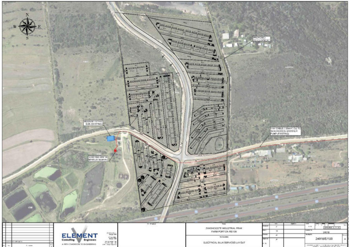
Figure 7: Bulk Electrical Services Layout
