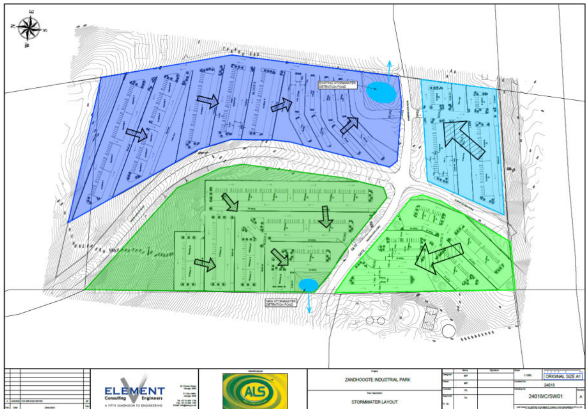
Figure 6: Preliminary stormwater drainage zones
