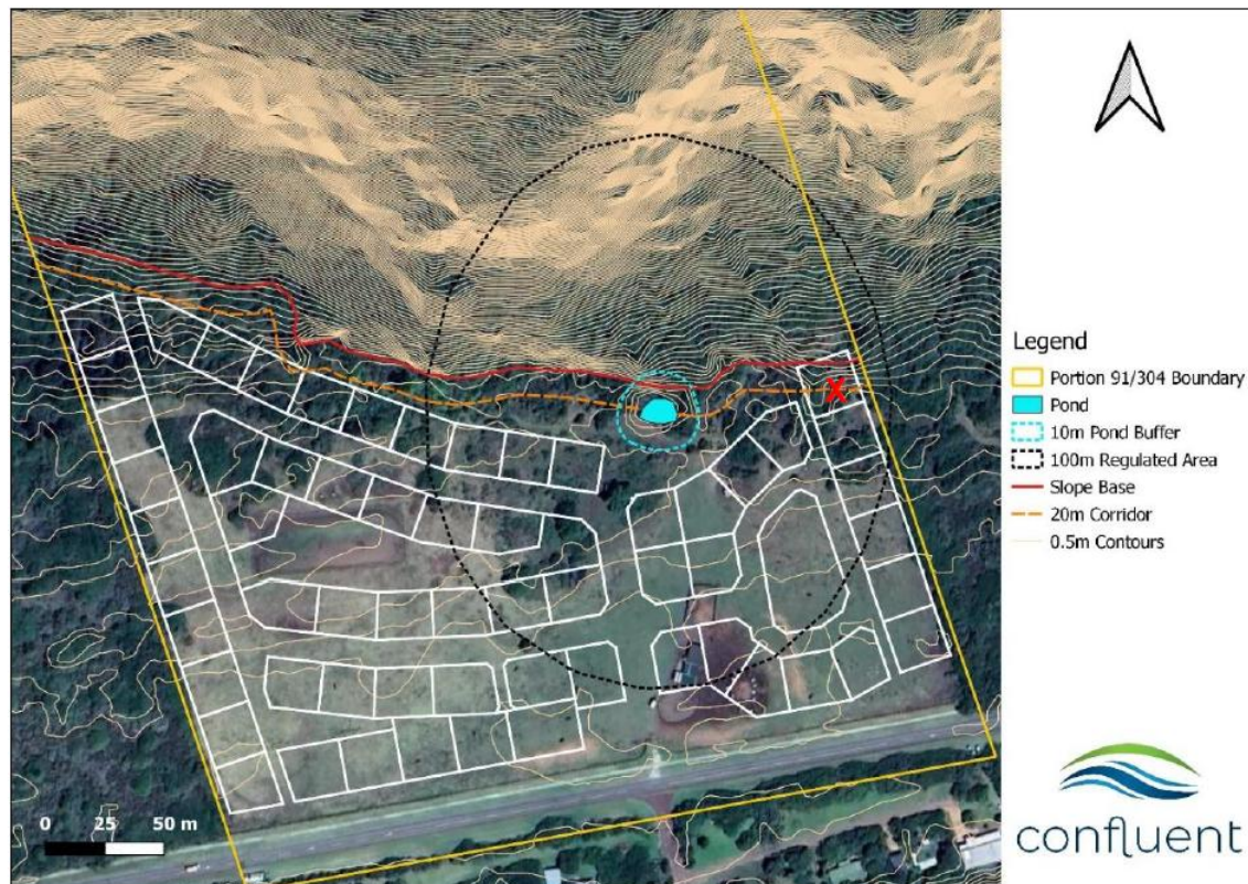
Figure 10: Preferred site development plan overlaid with 0.5 m contours, indicating the pond and buffer, the 100m regulated area of the spring, and the 20m wildlife corridor at the base of the slope. Note that the red X indicates Unit 50 which was subsequently moved back and out of the wildlife buffer (Confluent, 2025).
