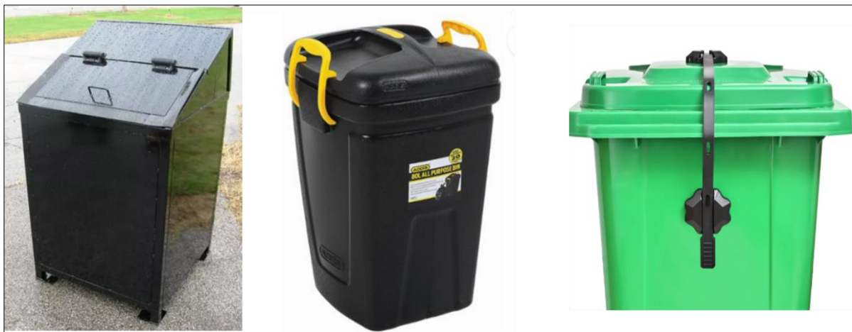
Figure 27. Wildlife-proof garbage disposal container options. Large containers with a one-way shoot to dispose of garbage (left): the top lid is connected to a smaller container which swivels up when the lid is opened to block access to the larger bin and its contents below, but when the lid is closed this bin swivels down to drop the garbage into the larger container. Locking mechanisms and handles on bins (middle and right) can also be used to successfully keep wildlife out.
