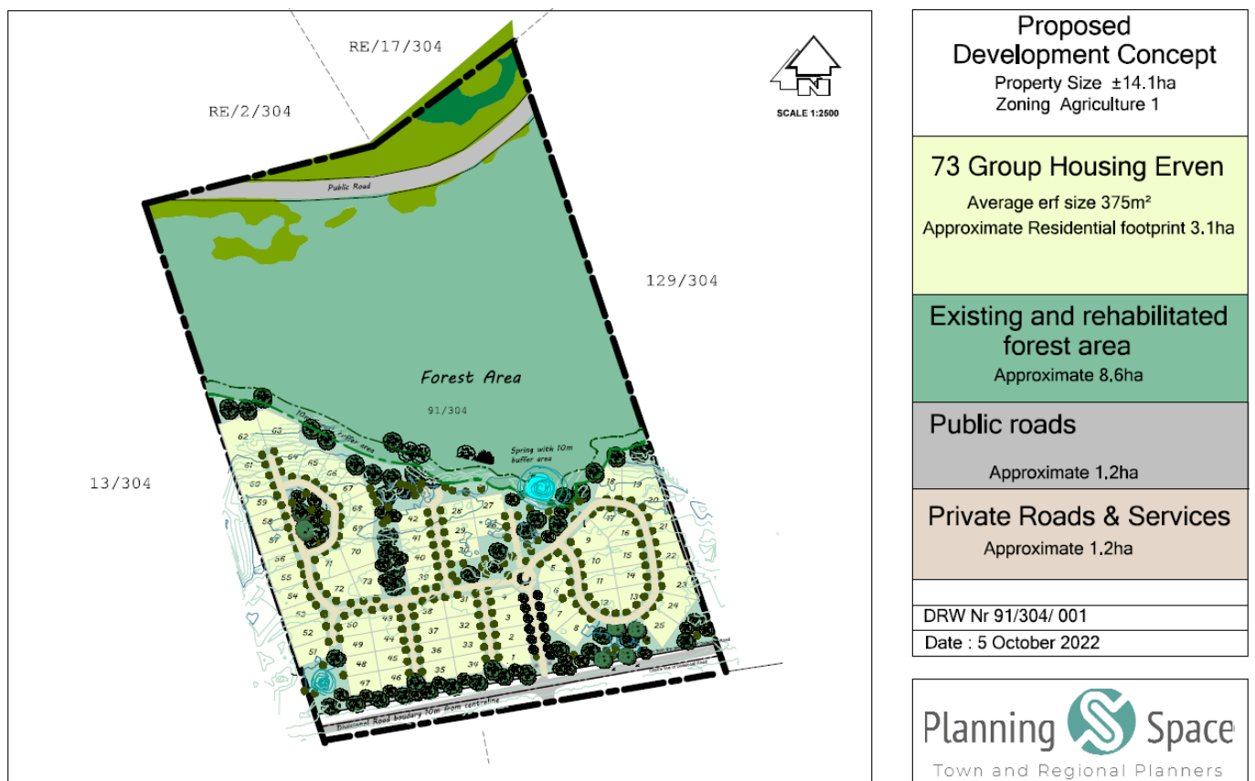
Figure 3: Layout Alternative 1 - \pm 73 group housing stands with average erf sizes of \pm 375\text{m}^2 .
