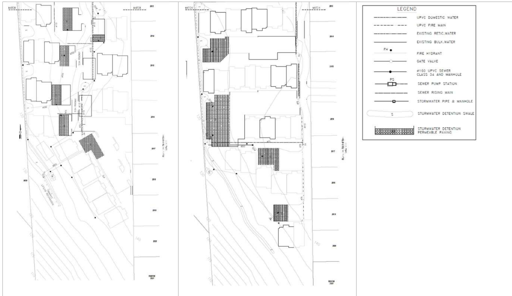
Figure 4: Proposed sewer and water reticulation, roads and stormwater layout for SDP Alternative 1 (left) and SDP Alternative 2 (right).
