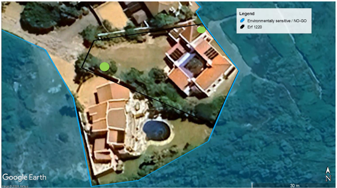
Figure 1: All open areas outside the erf are No-go areas; access to eastern areas must be restricted during construction; Milkwood trees (indicated in green) must be cordoned off prior to start construction.
