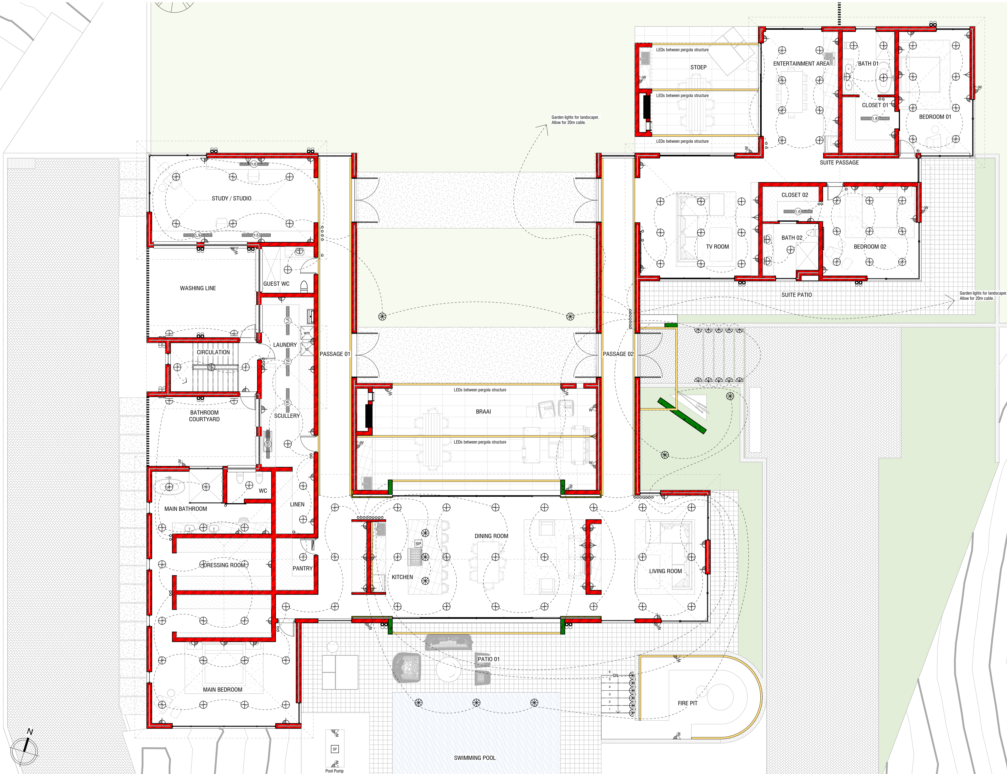
Ground - Electrical Plan
