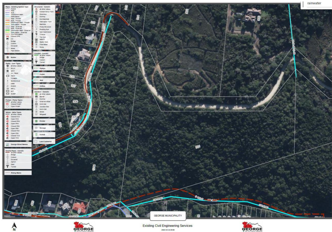
Figure 8: Existing Municipal services. 50mm diameter water connection (blue) and 160mm diameter sewer line (red dashed).
