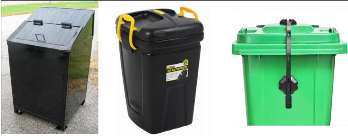
Figure 21. Wildlife-proof garbage disposal container options. Large containers with a one-way shoot to dispose of garbage (left): the top lid is connected to a smaller container which swivels up when the lid is opened to block access to the larger bin and its contents below, but when the lid is closed this bin swivels down to drop the garbage into the larger container. Locking mechanisms and handles on bins (middle and right) can also be used to successfully keep wildlife out.
