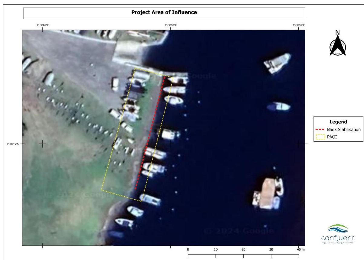
Figure 10: Map illustrating the extent of the streambank stabilisation and the associated PAOI.
