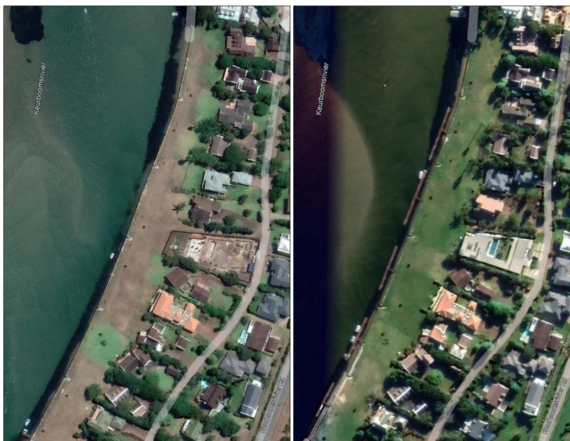
Figure 14: Google Earth images showing Z. capensis beds pre (left) and post (right) construction of bank stabilisation and floating jetties along the eastern bank of the Keurbooms Estuary.
