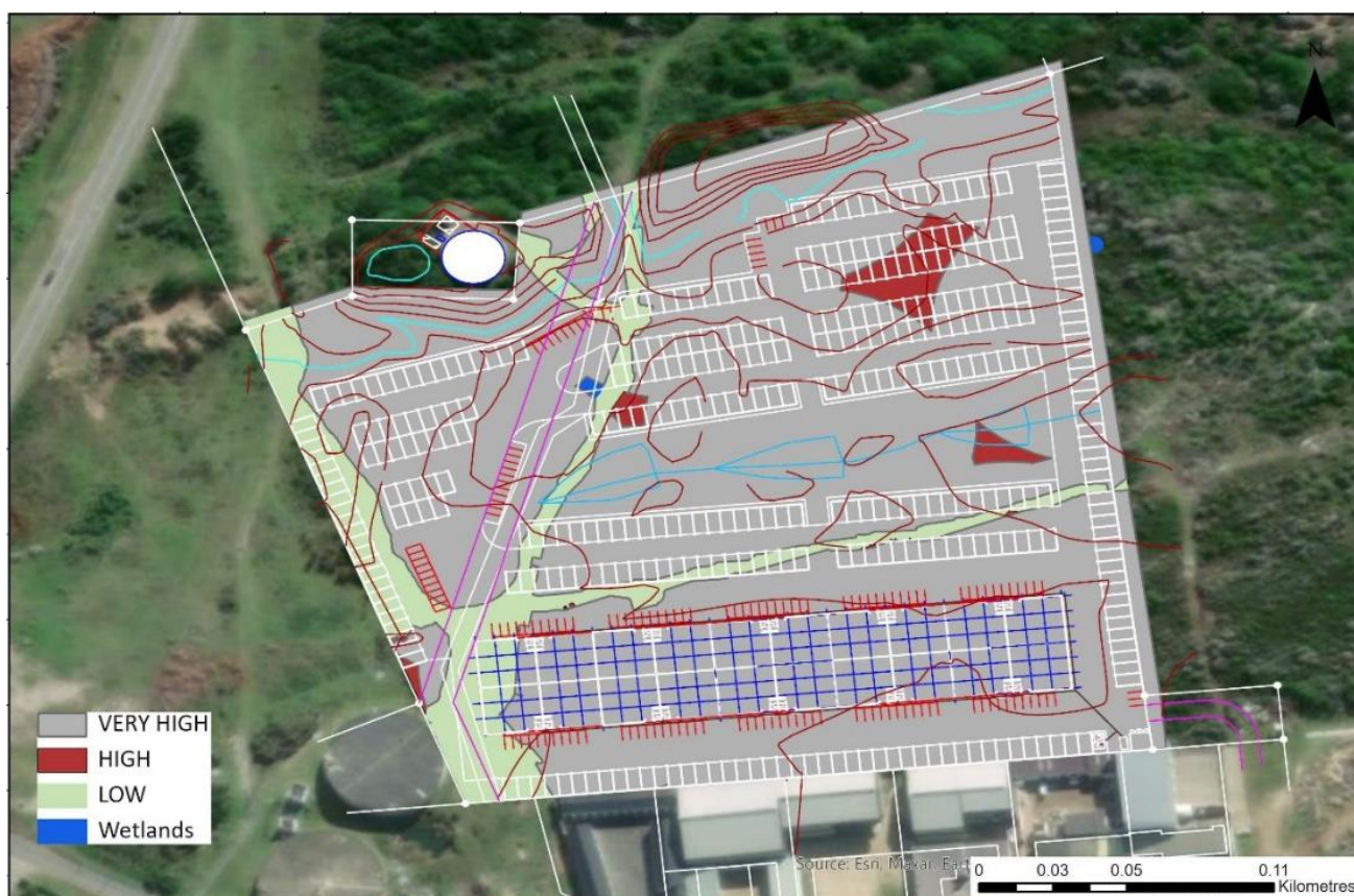
Figure 19: Sensitivity Map of the proposed Goedgeloof Warehouse and Storage Facility overlaid on Alternative Layout 2.
