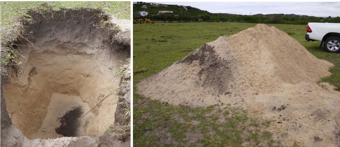
Figure 6: Typical sandy soil types encountered in test pits
