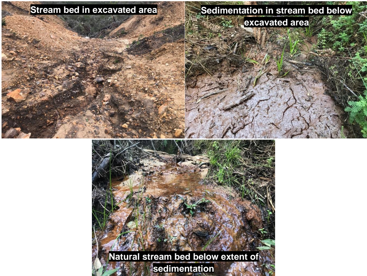
Figure 12. Stream bed in the excavated area, and downstream with / without sedimentation as labelled.
