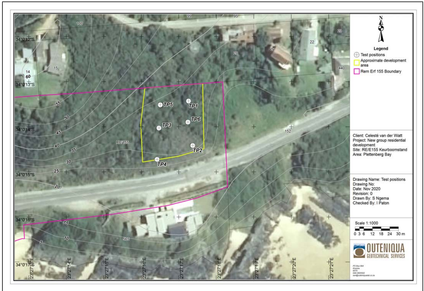
Figure 6: Plan of test positions
