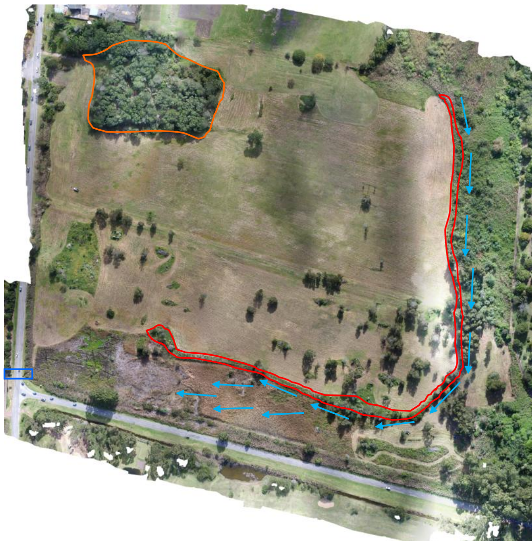
Figure 4. Aerial drone image (2018) of the George Rex Wetland showing degraded features. Blue arrows show the stormwater channel, the red area is the stormwater channel embankment, the orange area is the historical soil stockpile which has been colonised by alien trees (in the footprint of the sports complex), and all open areas are mown. The blocked culvert in the south-western corner is indicated by the blue rectangle.
