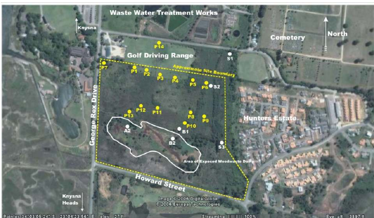
Figure 4.3: Location of water level sampling points and piezometers (WSP Environmental, 2006).
