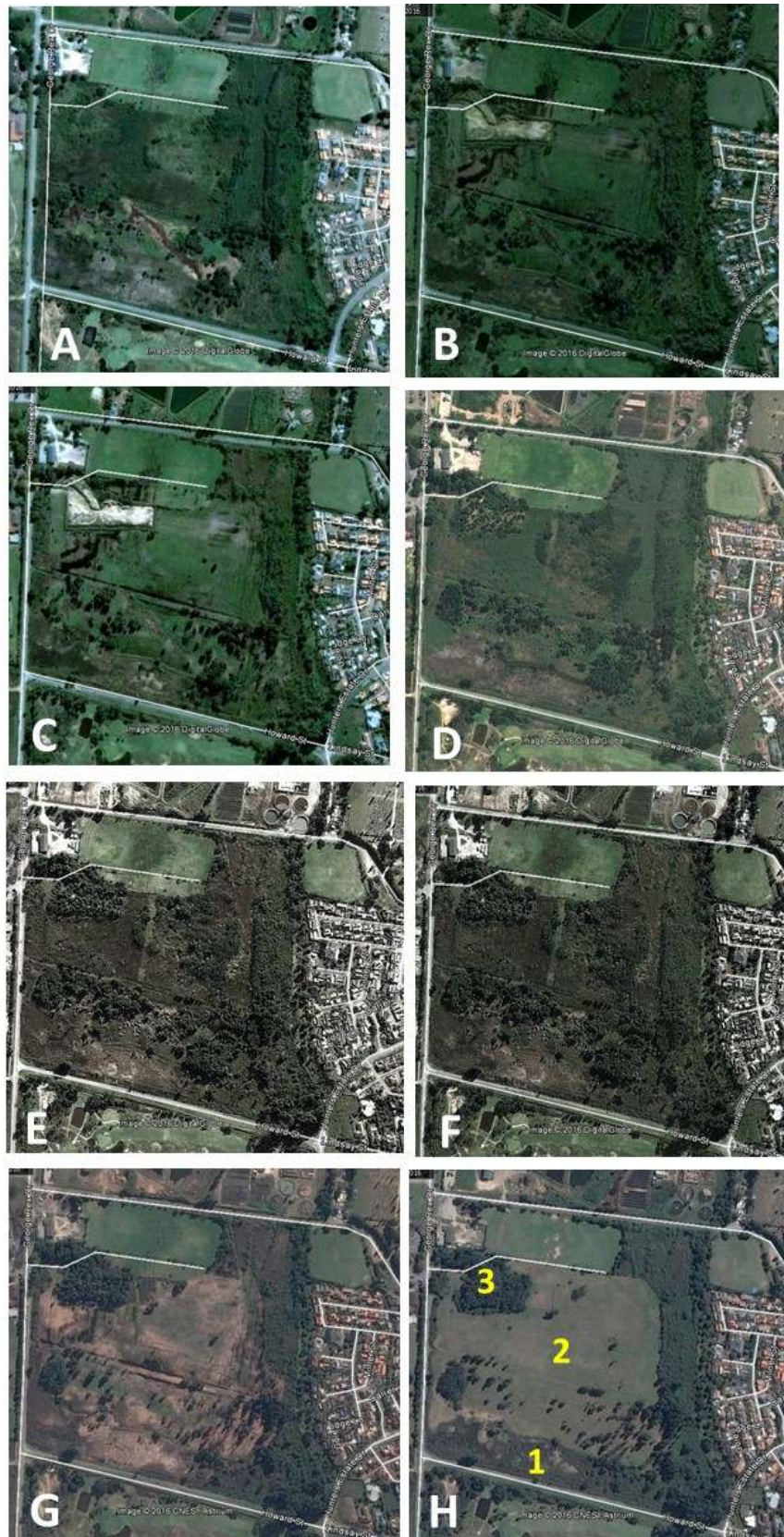
Figure 5.2: Google Earth images from 2003 (A), 2005 (B), 2006 (C), 2010 (D), 2011 (E and F), 2013 (G) and 2016 (H) that show the changing vegetation of the site through this period. In the 2016 image (H), the main vegetation types - reeds (1), mowed grass (2) and invasive alien trees (3) - are indicated.
